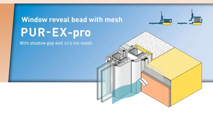
The APU window reveal bead with mesh PUR-EXpro is used in compound heat insulation systems as specified in the latest APU selection criteria. Within the reveal the profile is stuck flush to the structural element there and thus forms a clean and reliable termination of the plaster with shadow gap.
